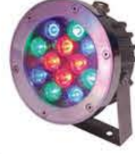
DS-G507 Size: Φ160*210mm Input Vol: AC/DC 12V Power: 12*1W Color: Single color/RGB Material: 304 stainless steel IP grade: IP68
