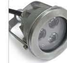
DS-G512 Size: Φ92*145mm Input Vol: AC/DC 12V Power: 3*1W/3*3W Color: Single color/RGB Material: 316 stainless steel IP grade: IP68
