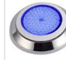
DS-G509/20W Size: Φ295*62mm Input Vol: AC/DC 12V Led Source: 105pcs 5050SMD Color: Single color/RGB Material: 304 stainless steel+PC cover IP grade: IP68
