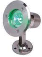
DS-G507 Size: Φ65*72mm Input Vol: AC/DC 12V Power: 1*1W Color: Red/Blue/Green/Yellow /White/Warm white/Pink/Purple Material: 304 stainless steel IP grade: IP68
