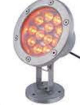
DS-G512 Size: Φ160*190mm Input Vol: AC/DC 12V Power: 12*1W Color: Single color/RGB Material: 304 stainless steel IP grade: IP68
